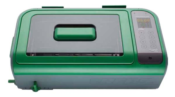
The new RCBS® Ultrasonic Case Cleaner-2 includes significant changes from the previous model. The Ultrasonic Case Cleaner-2 is larger - nearly 100 percent larger. The 6.3-quart capacity is twice as big, with a second ceramic heater and transducer to better clean brass cases and firearm parts. The LCD is easily programmable, and the timer can be set for up to 30 minutes of continuous cleaning. The Ultrasonic Case Cleaner-2 delivers clean brass in a short amount of time.
